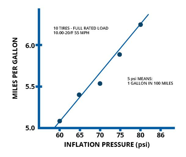
If the tires were an average of twenty pounds low when the tires would have been 95 pounds, the company would loose 50% of the tire wear. On the other hand, the twenty pounds of air pressure will cost more than double the amount of tires wasted in dollars but obviously not in percentage of fuel costs.
