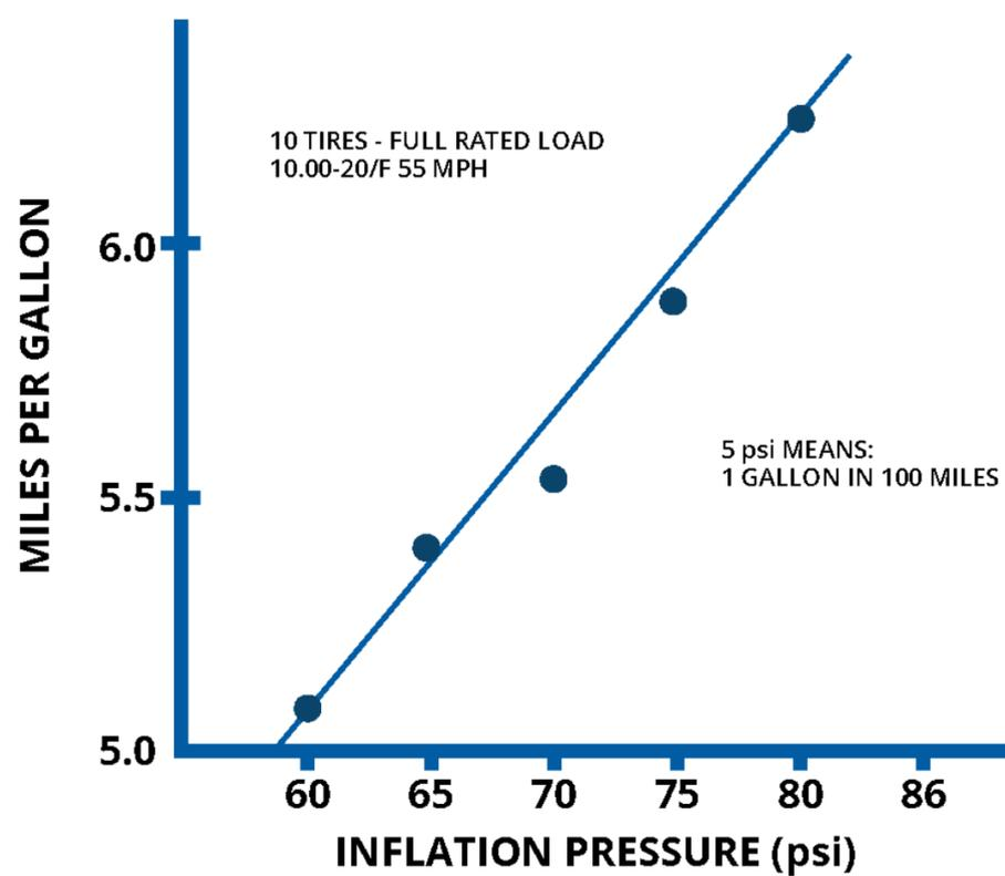
If the tires were an average of twenty pounds low when the tires would have been 95 pounds, the company would lose 50% of the tire wear. On the other hand, the twenty pounds of air pressure will cost more than double the amount of tires wasted in dollars but obviously not in percentage of fuel costs.
