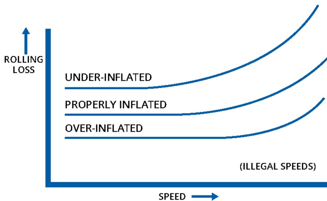
Over-inflation can also be devastating, but to a lesser degree than under-inflation. If over-inflation is severe, the tire can cause the rim to separate. This is extremely dangerous. Increasing inflation pressures will increase the load-carrying capacity of the tire up to a certain point, which is listed on the side of the tire. Over-inflation tires also cause tire damage due to the fact that the tire is unable to absorb shock. Slight over inflation can result in fuel savings.
